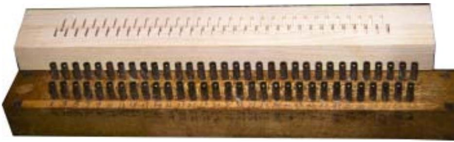
**Al Pohlpetter** is constructing a tracker bar (shown partly constructed at left, upper) based on the original (left, lower) for a Wurlitzer Automatic Harp. Al says there are only 20 of these harps in existence.
