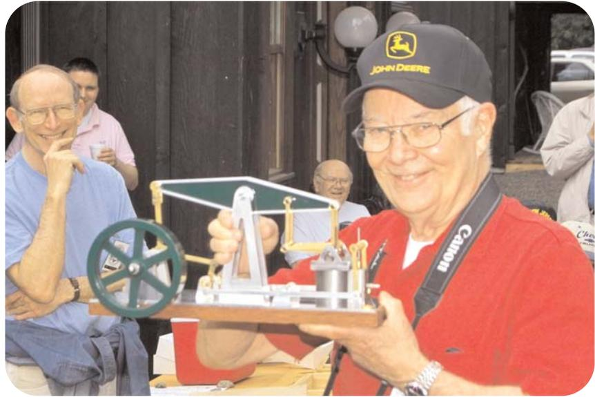
Still another own designed CNC milled project is that of **Bill Miller's** (shown below). This novel gas engine uses the Atkinson cycle linkage to attain 4 cycles (intake, compression, power and exhaust) in just one complete cycle of the piston. A particularly novel aspect of this design is the use of the drive shaft as intake and exhaust ports. Wow. Looks like this might make a good article for Home Shop Machinist.
