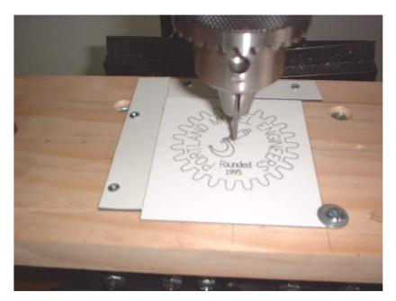
Bill Miller and Pat Wickers showed off their CNC mill conversion by creating new PME badges. The whole assembly is driven by a surplus '486 which was otherwise gathering dust; making the setup quite portable. Some ingenious work was done to create a zero-backlash nut for the leadscrew out of Delrin.
