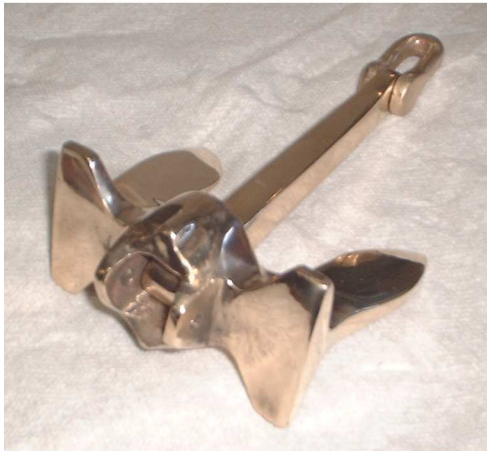
Bud Statton showed how his anchor project has turned out. The castings came back from the shop and were buffed to a high polish finish.
