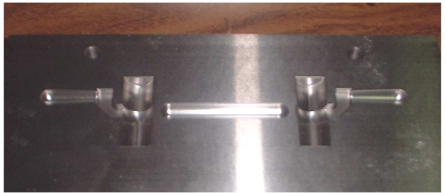
Hans Strangier and Grant Carson showed some steel dies that they produced. The die on the left includes bearing covers while the one on the right has two brake handles.
