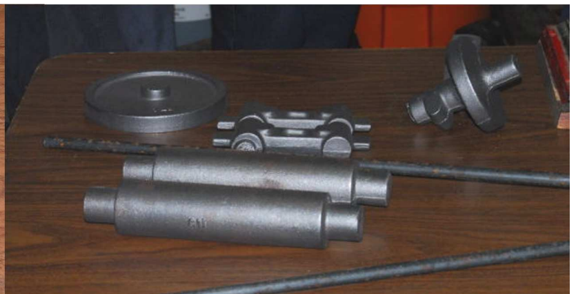
Gary Martin talked about the pillar tool featured in the book "Workshop Techniques" and showed some of the castings for the tool. Both this book and "The Model Engineer's Workshop Manual" by the same author are highly recommended reading.
