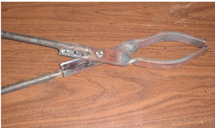
Wes Ramsey whipped together these crucible tongs from scrap he had laying around.
