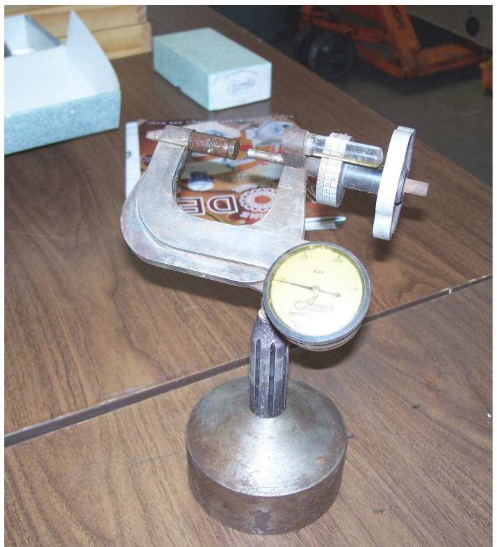
Carl Peterson brought in what appears to be a micrometer on a stand. It turns out to be an Ames hardness tester.
