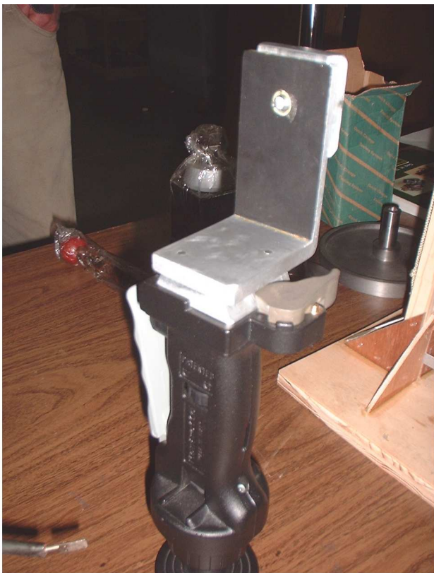
Above Vince Kurpan demonstrated his answer to the problem of handling a heavy camera on the end of a tripod. It has a quick disconnect to transform from horizontal to vertical.
