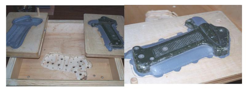
Bud Statton explained how to do no-bake molding. The green section is the handle to his Vietnam era flamethrower. The grey portion is the material necessary to raise the parting line to match the part. No-bake is quite a bit more expensive than greensand casting but does have the advantage that the mold doesn't suffer from dropout.
