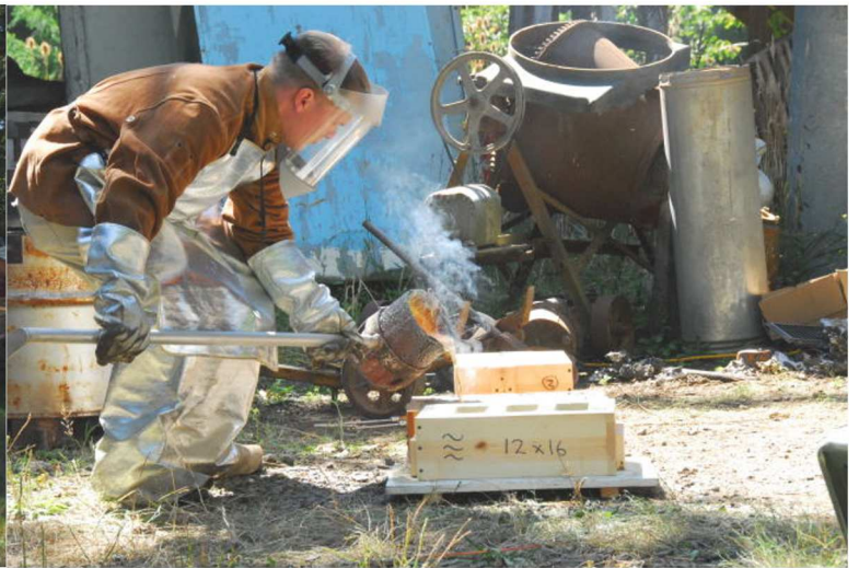
On the left, Bud Statton explains the finer points of casting. To the right, Jarod Eells pours a full crucible of brass into the mold.
