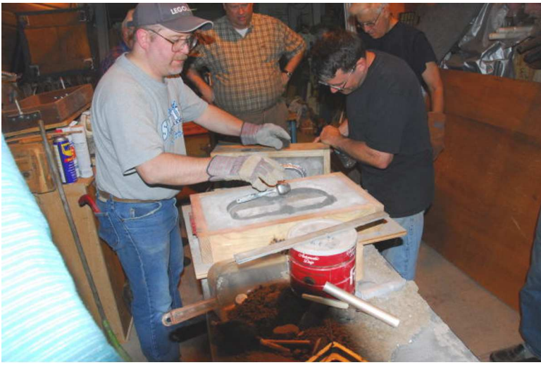
Bill Baker and Gary Martin worked on ramming a pattern for a machinists level. On the right, are two of Bill's castings for spoke shaves in brass that had just come out of the sand.
