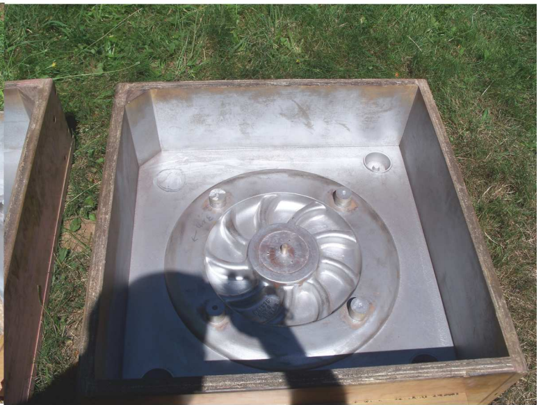
Gary Martin brought a pattern for railroad wheels destined for Disneyland. The walls on the sides of the pattern indicate that they will be done in "no-bake" sand which has a resin included in the sand. Below are patterns for a large hoist. You can see the lettering "RopeMaster" on the right side.
