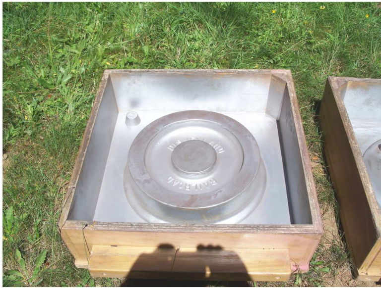
Gary Martin brought a pattern for railroad wheels destined for Disneyland. The walls on the sides of the pattern indicate that they will be done in "no-bake" sand which has a resin included in the sand. Below are patterns for a large hoist. You can see the lettering "RopeMaster" on the right side.
