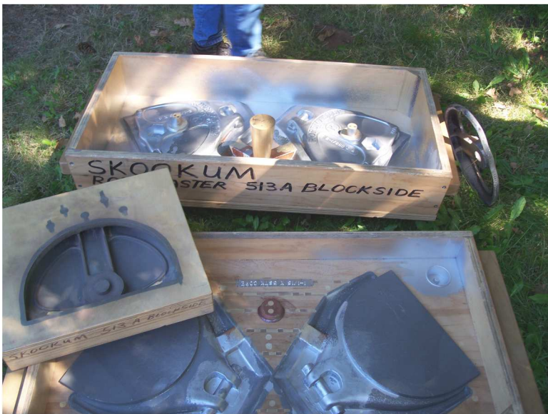
Gary Martin brought a pattern for railroad wheels destined for Disneyland. The walls on the sides of the pattern indicate that they will be done in "no-bake" sand which has a resin included in the sand. Below are patterns for a large hoist. You can see the lettering "RopeMaster" on the right side.
