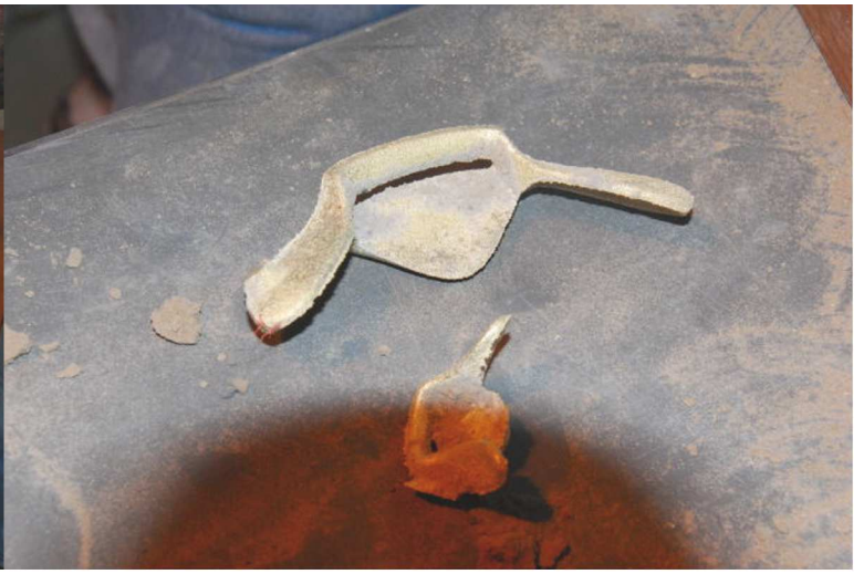
Bill Baker and Gary Martin worked on ramming a pattern for a machinists level. On the right, are two of Bill's castings for spoke shaves in brass that had just come out of the sand.
