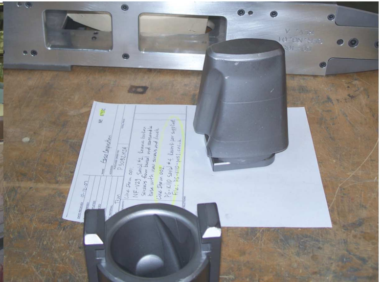
Those of us who took the Columbia Steel foundry tour will remember seeing parts made from this pattern. The teeth on the large buckets rapidly wear off and need to be replaced.
