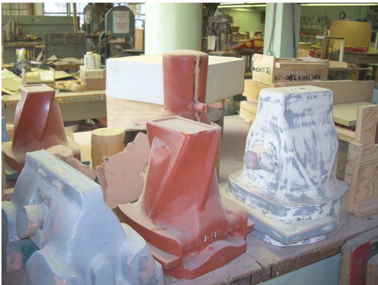
Those of us who took the Columbia Steel foundry tour will remember seeing parts made from this pattern. The teeth on the large buckets rapidly wear off and need to be replaced.
