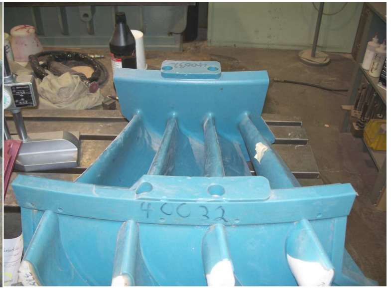
Here are two examples of patterns for gas turbine blades that were cast in wax. The white material is a core which will make the vanes hollow. Small changes of mere thousands of an inch affect balance and performance.
