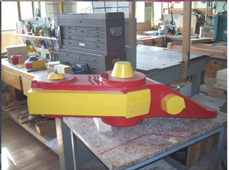
These patterns are used to form core prints for the larger pattern on the right. The cores help to keep metal cross-section to a uniform thickness and reduce the overall weight of the piece.
