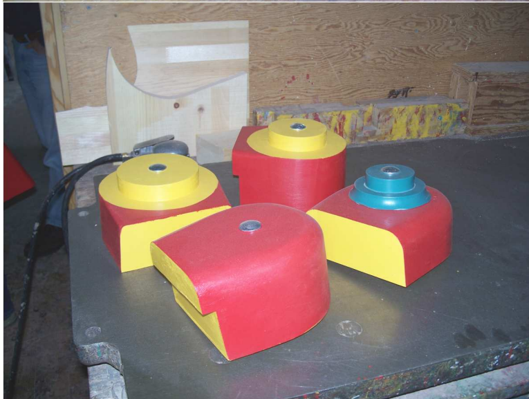
These patterns are used to form core prints for the larger pattern on the right. The cores help to keep metal cross-section to a uniform thickness and reduce the overall weight of the piece.
