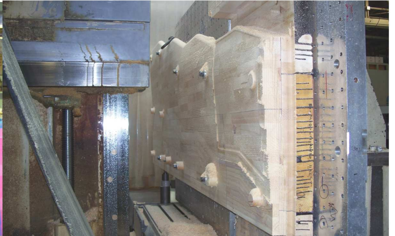
A large 3D CNC router in action carves a part out of a 10 foot section of glued-up planking.
